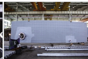
1ST SHELL NOZZLE & MANHOLE
